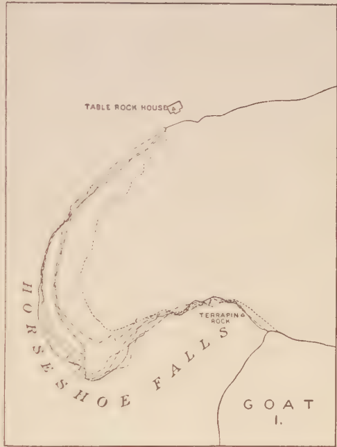
FIG. 573. Outline map of a portion of the crest line of Niagara Falls, showing the recession of the brink during various intervals since 1842. (After Taylor.)
